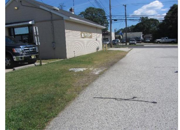
A bioretention system can be implemented in the turfgrass area adjacent to Lester Avenue to manage stormwater from the street, rooftop, and parking area. Bioretention systems are green infrastructure practices designed to capture, retain, and infiltrate stormwater. A preliminary soil assessment suggests that the soils have suitable drainage characteristics for green infrastructure.
