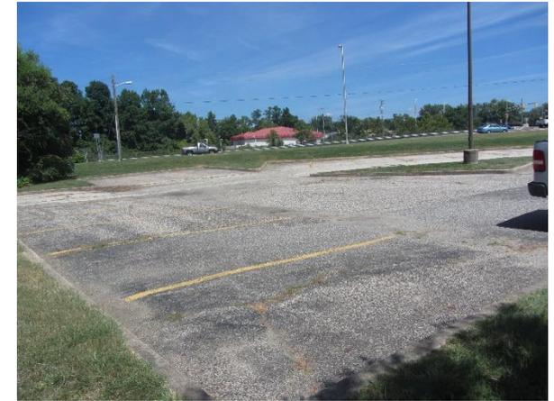
The parking spaces in the northern end of the parking lot can be replaced with porous asphalt to capture and infiltrate stormwater. Due to the slope of the lot, the parking spaces can collect stormwater from other sections of the lot as well. A preliminary soil assessment suggests that soil testing is needed to determine if the site has suitable drainage characteristics for green infrastructure
